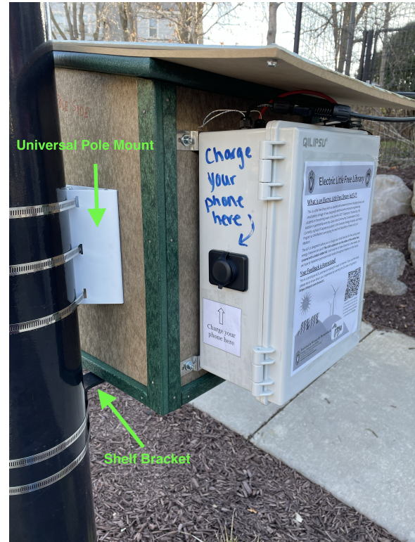
(b) Prototype showing the Universal Pole Mount and the Shelf Bracket
